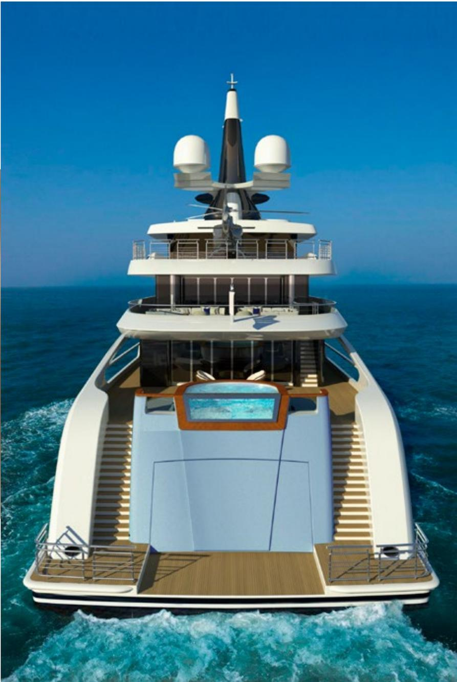
This is now an essential feature on yachts this size. Because the aft door folds down instead of up we created a large platform and beach club with minimum shade and a feeling of light. This is helped with a skylight in the bottom of the pool.
